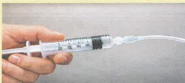
1. Attach Teflon Tube to Syringe
