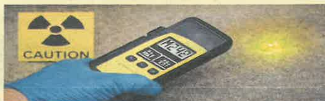
1. Detect Hot Spot with Radiation Detector
